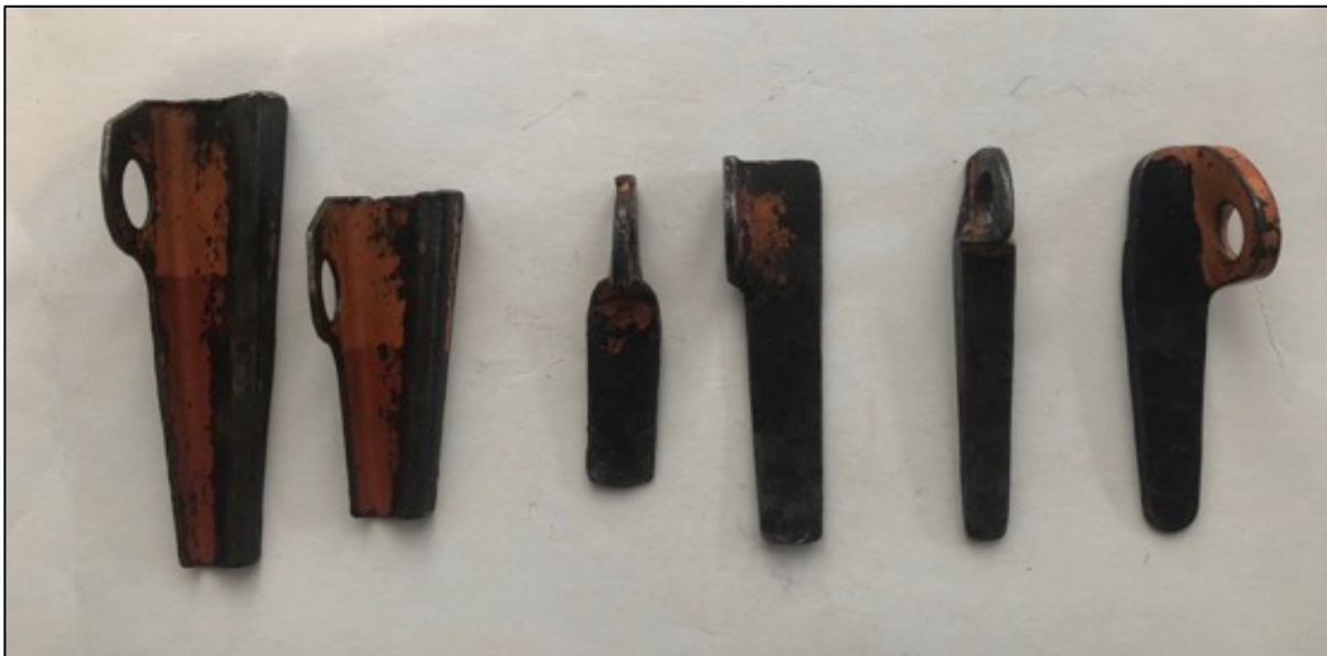
Chrome-moly pitons. From left to right: two Leepers (made by Ed Leeper), two Chouinards and two Clogs (UK).
