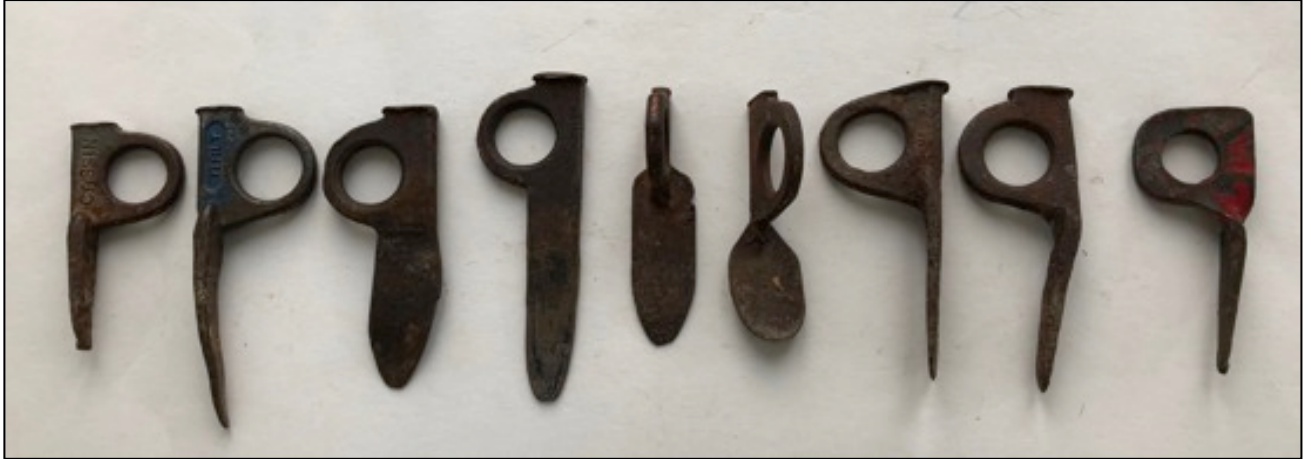
Eight European soft steel pitons by Cassin and Stubai and, on the far right, a hard steel piton made by Stuart Fishwick. George Adams collection.
